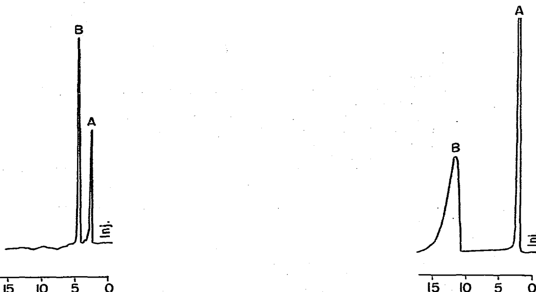
Fig. 2. Liquid chromatogram of Acacia podalyriaefolia leaf extract. A = Solvent impurity; B = tryptamine.
